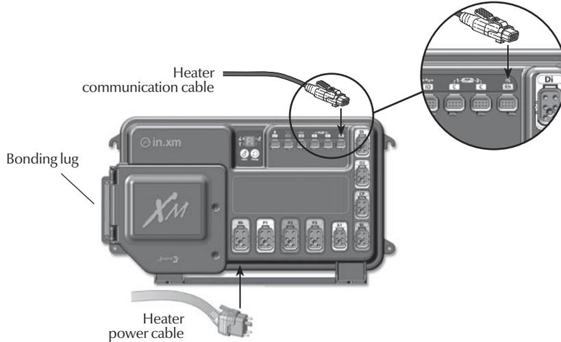
Connect the heater power cable to the in.link output connector indicated Rh on the spa pack.
