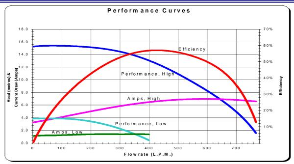
These performance curves are a result of in-lab testing, actual performance may vary based on manufacturing tolerances and application.
